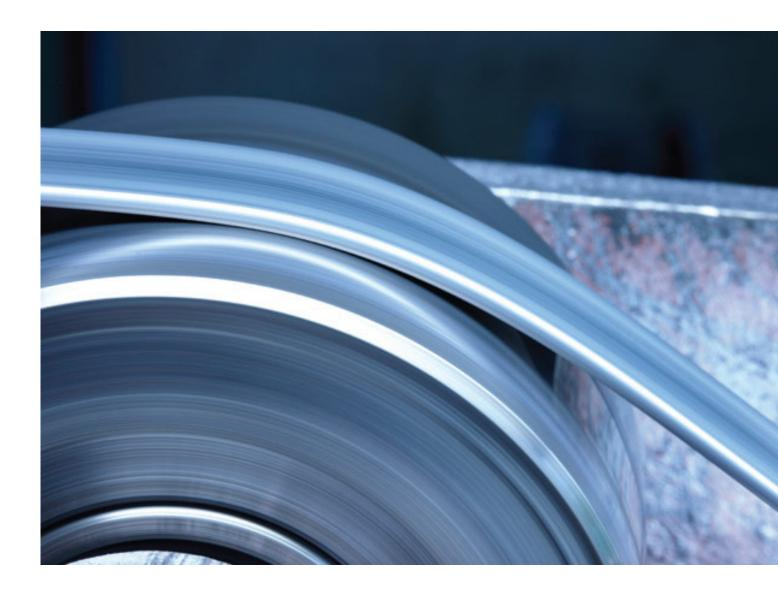
The flanging process allows you to have a round edges, removing the excess burr and maintaining the width and thickness tolerances unaltered. We can obtain strips, oscillated strips and flanging strips.
