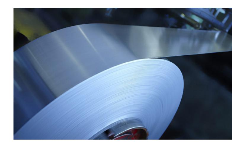
It is a mechanical process that permits decreasing the thickness of the material by passing it through cylinders with a distance between them that is less than the original thickness. The material subjected to this crushing undergoes an internal stress that strengthens it by hardening it and guaranteeing a tighter tolerance than required by current standards.
